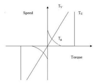
Component Tv varies linearly with speed is called VISCOUS friction and is given by
